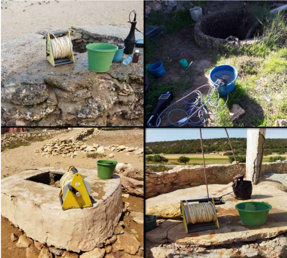
Figure 5. Examples of some wells measuring piezometric level
