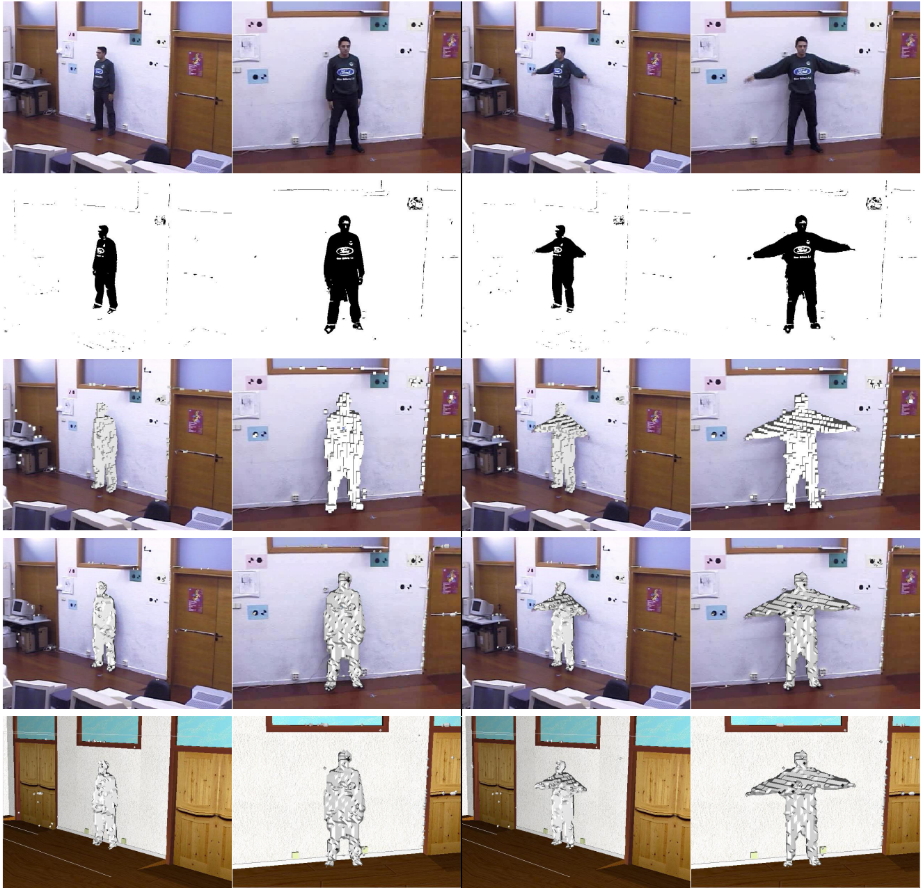
Fig 2. Two frames, left frame number 190, right frame 250 from two color cameras. Top to bottom: real image, segmentation, voxel representation, marching cubes rendered image, and virtual world mixed marching cubes
