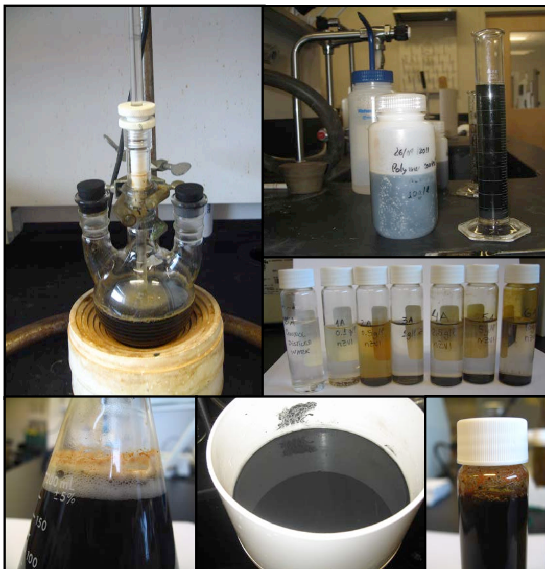
Figure 1 – different aspect of the laboratory synthesis of zero-valent iron nanoparticles.
