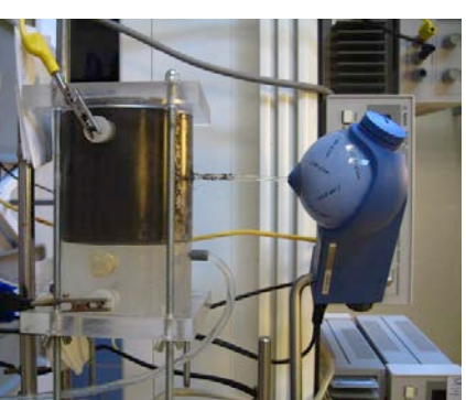
d) Two compartment Electroalytic setup used with PCB contaminated soil (DTU).
