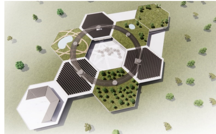
Figure 2. A top view of the design of the school fully energy self-sustainable with photovoltaics.
