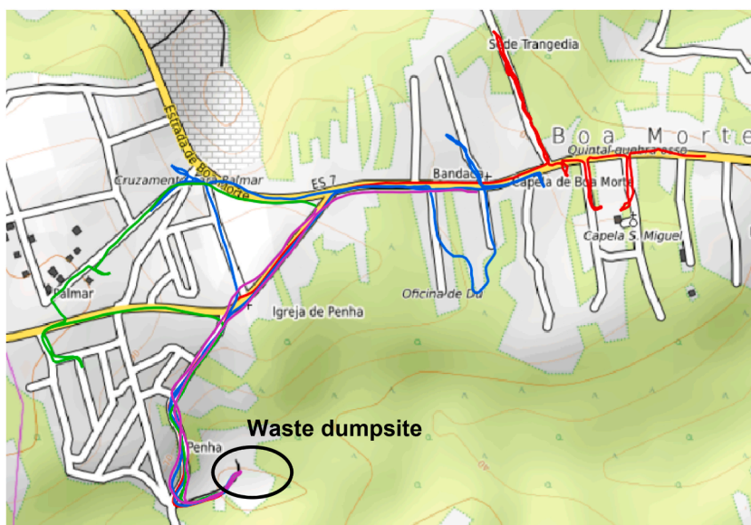
Fig. 10. Representation on a map of a geo-referenced recording of the collection route in Boa Morte. Each colour represents an itinerary: red is itinerary 1 (7 collection points), blue is itinerary 2 (8 collection points) and green is itinerary 3 (3 collection points), plus the final return (purple); adapted from ©OpenTopoMap (CC-BY-SA). (For interpretation of the references to colour in this figure legend, the reader is referred to the Web version of this article.)
