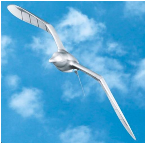
Figure 1.1.2. SmartBird flies like a bird (FESTO).
