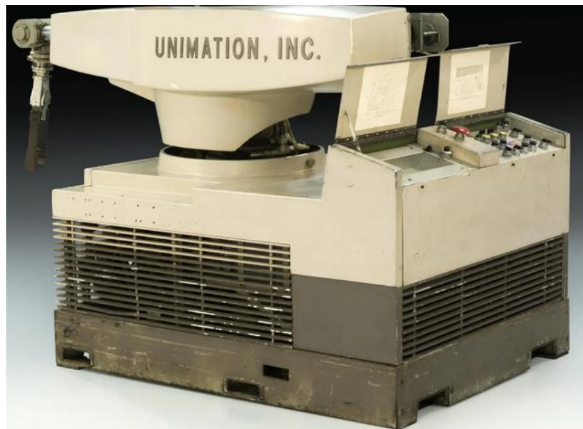
Figure 1.1.9. Unimate, the first industrial robot (IEEE Spectrum).
