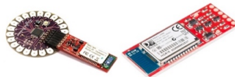
Fig. 212 - LilyPad Arduino com SparkFun Bluetooth Mate Gold e SparkFun Bluetooth Mate Silver 275 .
