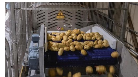
Potato outlet of an industrial PEF system in a French fry processing line. (Elea GmbH 2020)
