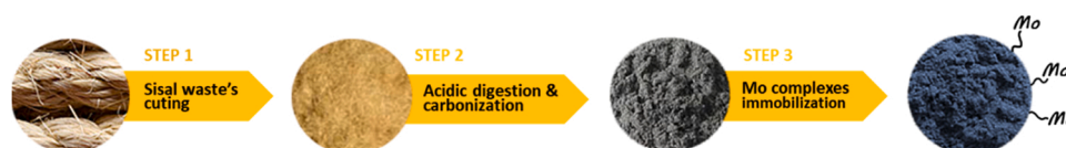
Fig. 1. Summary of steps for catalyst manufacturing: from sisal rope production waste to immobilized Mo complexes catalyst.
