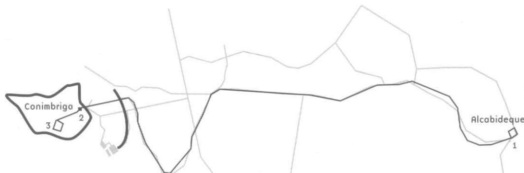
Conimbriga water mill. Path of the water from the spring to the forum, with the approximate location of the water wheel (in GORGES, 1997). 1 - Alcabideque spring; 2 - distribution chamber; 3 - baths to the south of the forum. (above) Photo which shows, on the left, marks of the vertical wheel on the gallery wall (Photo Museu Monográfico de Conimbriga , in GORGES, 1997).
