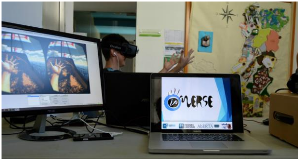
Figure 4 - Oculus Rift and Leap Motion combination, enabling the helmsman to see virtual renderings of arms and hands.
