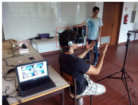
Figure 1 - Players using the prototype: Player 1 is sitting and using an Oculus Rift; Player 2 is standing in front of a Kinect 2 and moving his arm to control the Adamastor giant.
