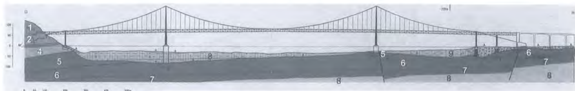
Fig. 9.2 – Geological section of the Tagus estuary. From Almeida, 1986. 1 – Quinta do Bacalhau sandstone; 2 – Forno do Tijolo clays; 3 – Entrecampos limestones; 4 – Estefânia clayey sandstone; 5 – Prazeres clays and limestones; 6 – Lisbon Volcanic complex; 7 – limestones; 8 – Clayey limestones and clays; 9 – Alluvial deposits.
