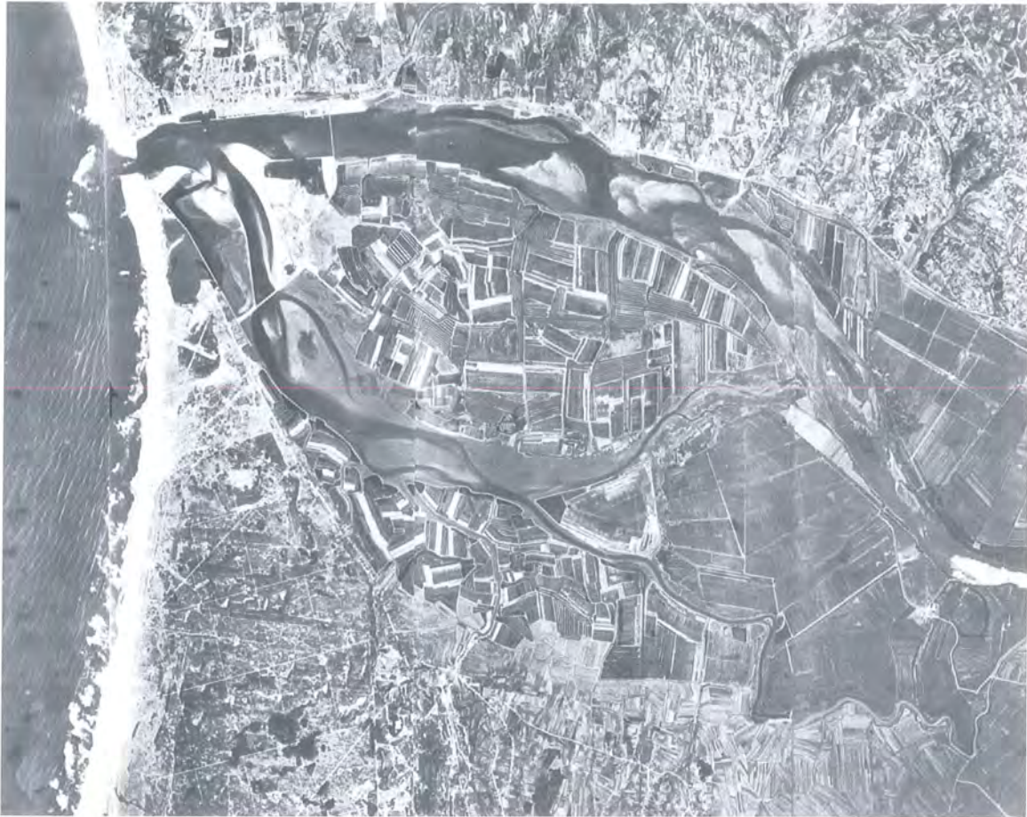
Fig. 5.6 – Mosaic of vertical aerial photos of the Mondego estuary (comprising the 9 km downstream) in a spring low tide of 1947 (summer). The human interventions were reduced and limited to the mouth area. Notice the general silting of both estuarine branches.
